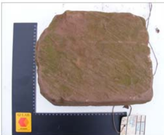
Plate 7, Stone 7, Dressed bedding plane and 6cm chamfer on the corner angle (at bottom left of picture).
