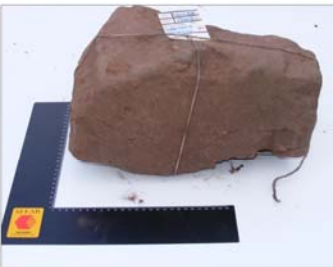
Plate 12, Stone 5, dressed face with tidy, tightly spaced tooling. Possibly dressed using a 2" (5cm) bolster.
