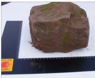
Plate 11, Stone 10, shows rough tooling on this end of the block, this appears to have been done using a 2½" (6.5cm) bolster.
