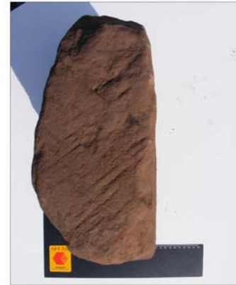
Plate 6, Tool marks on one end of Stone 8, The tooling is at 45°, but cutting from two directions has produced a chevron effect.
